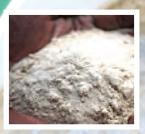
Ten tons of sand are contained within the treatment process. Silica microsand has a diameter of about 85 microns.
