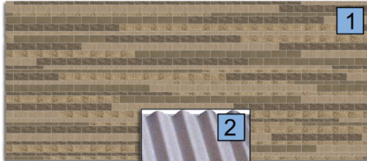
VARIED MASONRY WITH SPLIT & SMOOTH, 8x8x16 & 4x8x16, COLOR: WESTERN BROWN & JAVELINA BROWN
