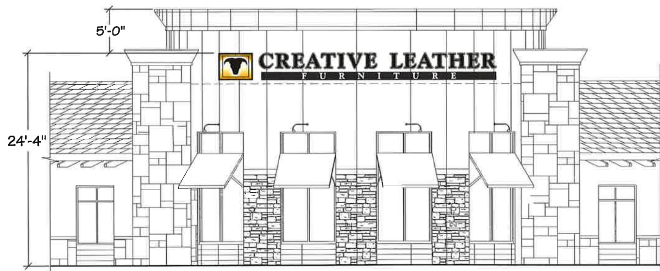
CL-1 PARTIAL SOUTH BUILDING ELEVATION SCALE: 3/32" = 1'-0"
