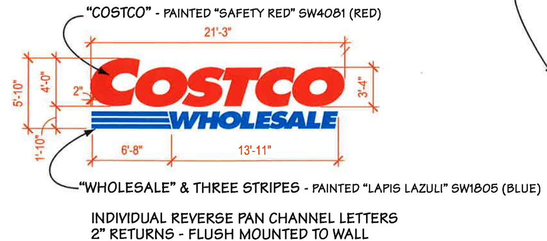
2. BUILDING SIGN C3 SPECIFICATION - SCALE: 1/8" = 1'-0"
