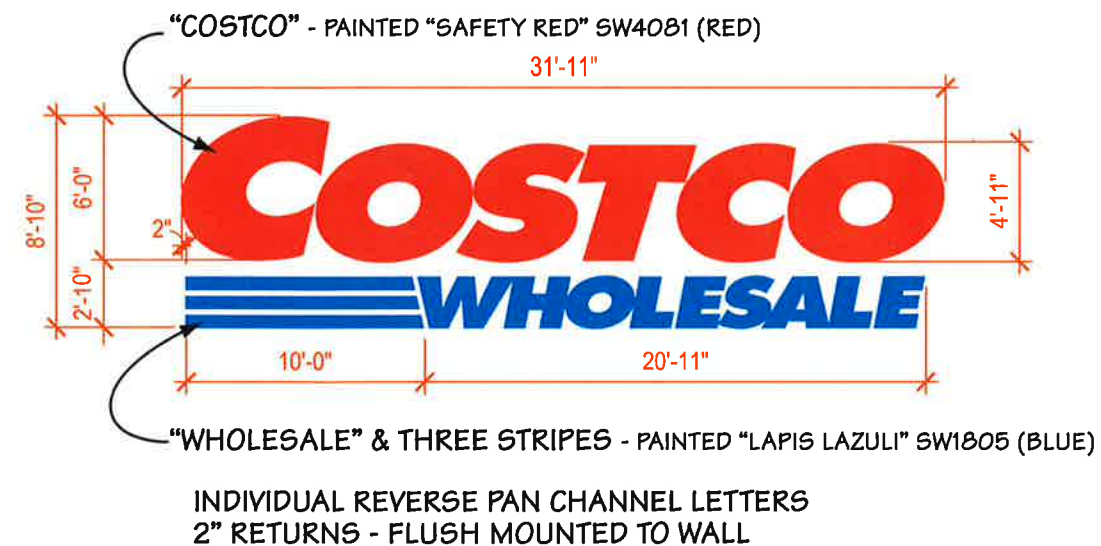
2. BUILDING SIGN C1 SPECIFICATION - SCALE: 1/8" = 1'-0"
