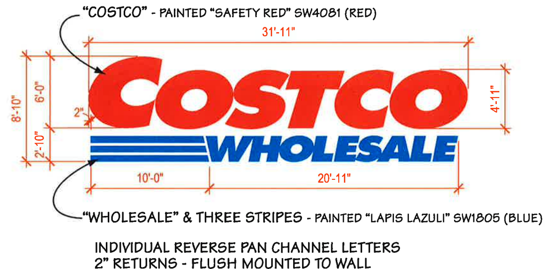
2. BUILDING SIGN C4 SPECIFICATION - SCALE: 1/8" = 1'-0"
