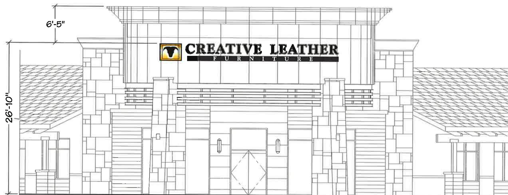
CL-2 PARTIAL NORTH BUILDING ELEVATION SCALE: 3/32" = 1' - 0"
