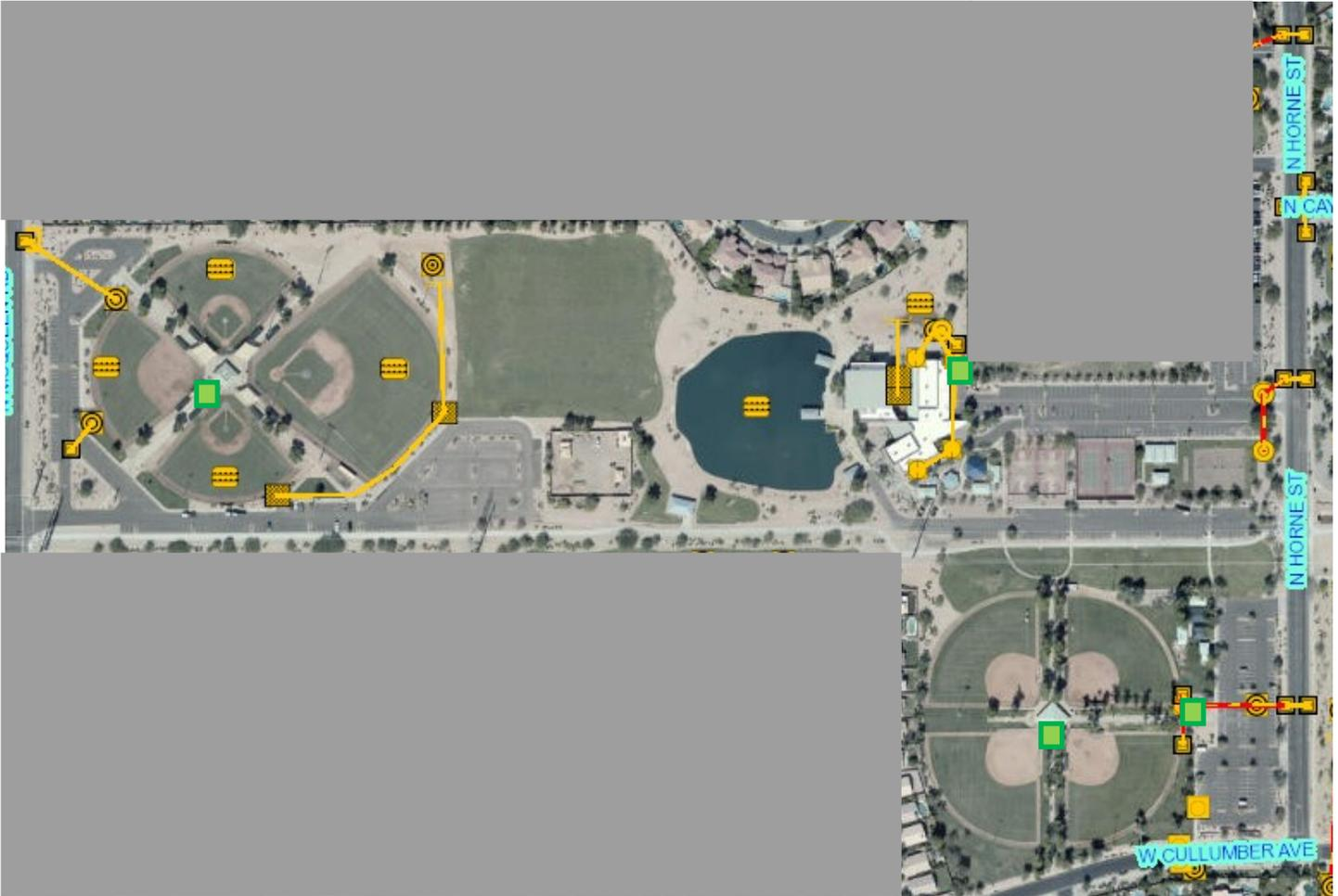
This map demonstrates the stormwater infrastructure that is potentially impacted. Utilize the contacts on the previous page to resolve issues in these areas. The symbols below are used to indicate hazardous material hot spots.
