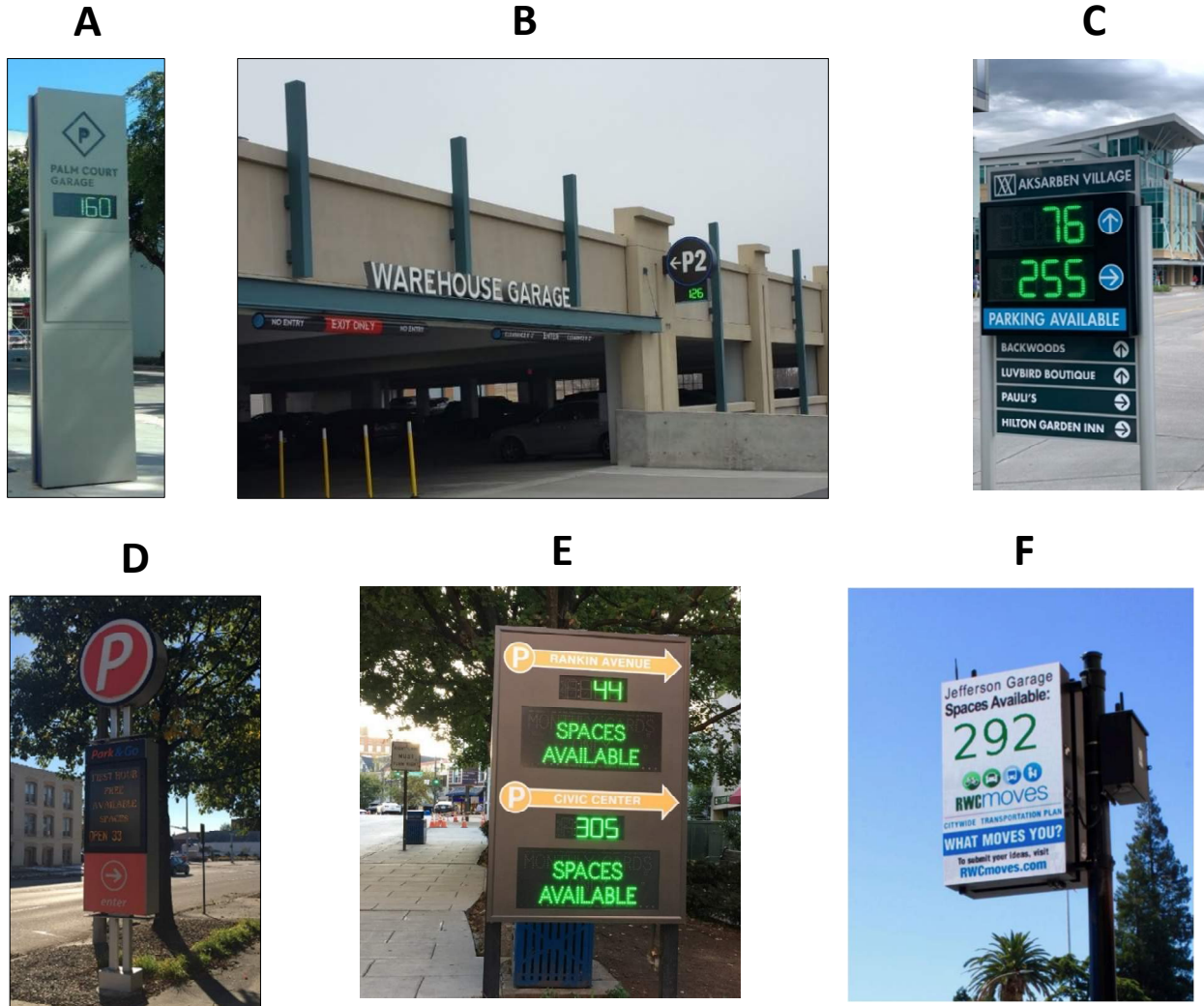
Figure 47: Examples of Facility-Status Type Guidance Signs
