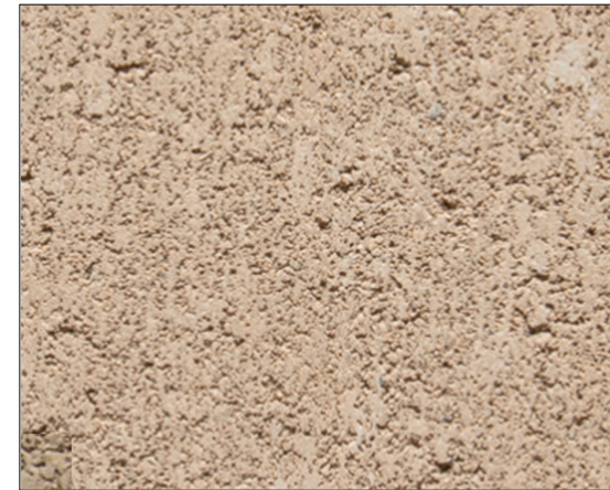
SPLIT FACE CMU COLOR: STAIN TO MATCH SUPERLITE NW BONE (OR EQUAL)
