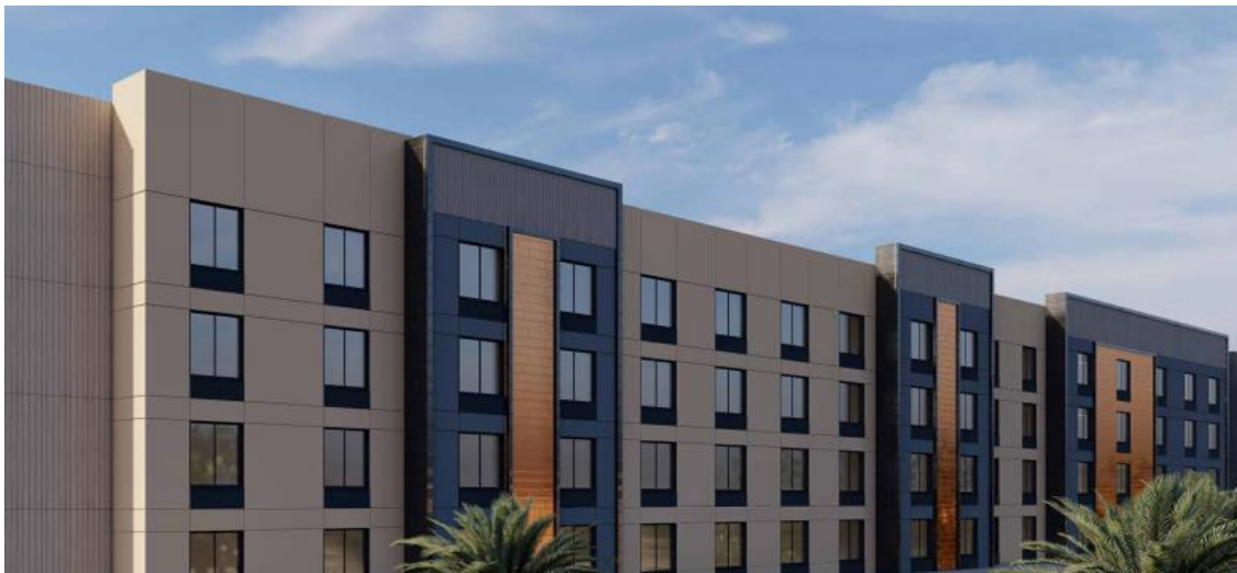
Figure A: A rendering illustration inset demonstrating how accent masses (dark grey-blue) relate to the rest of the structure. Note how rooflines of accent masses do not return into the main building. See comments above.
