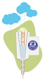
Place the rain gauge outside on a level surface, away from any overhanging eaves or trees. You may place the rain gauge directly in the ground or construct a simple stand to elevate the gauge above the ground. Leave the rain gauge outside for the entire school year.
