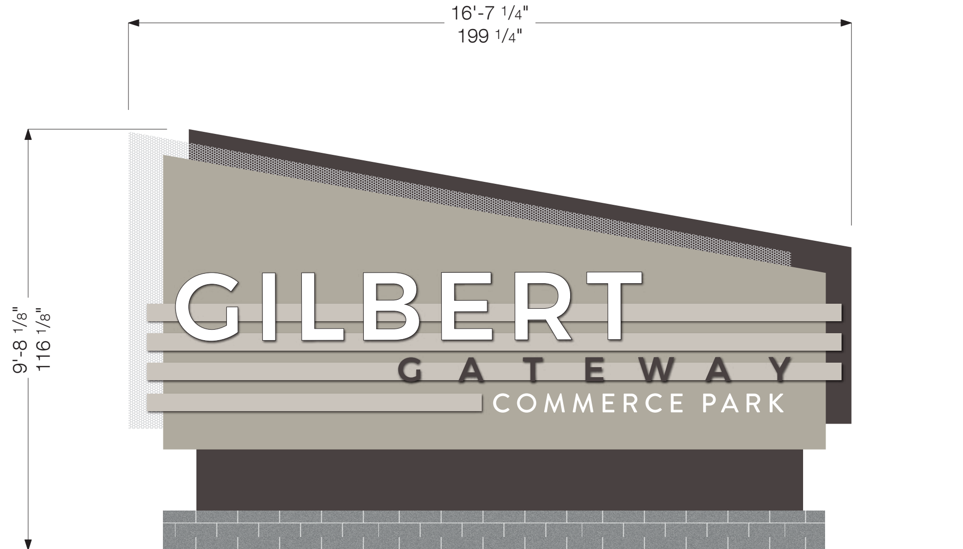
B Entry Monument | Elevation Detail SCALE: 1/4" = 1'
