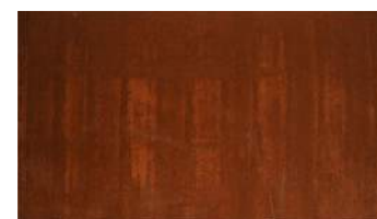
C6 Faux Rust Chemically activated rust finish applied to a common material
