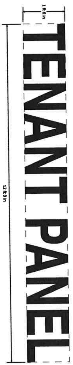
OPTION 1 Scale: 3/4" = 1' FABRICATE AND INSTALL REVERSE PAN CHANNEL LETTERS NON-ILLUMINATED 1" TO 2" DEEP LETTERS PAINTED MAP BLACK N-923
