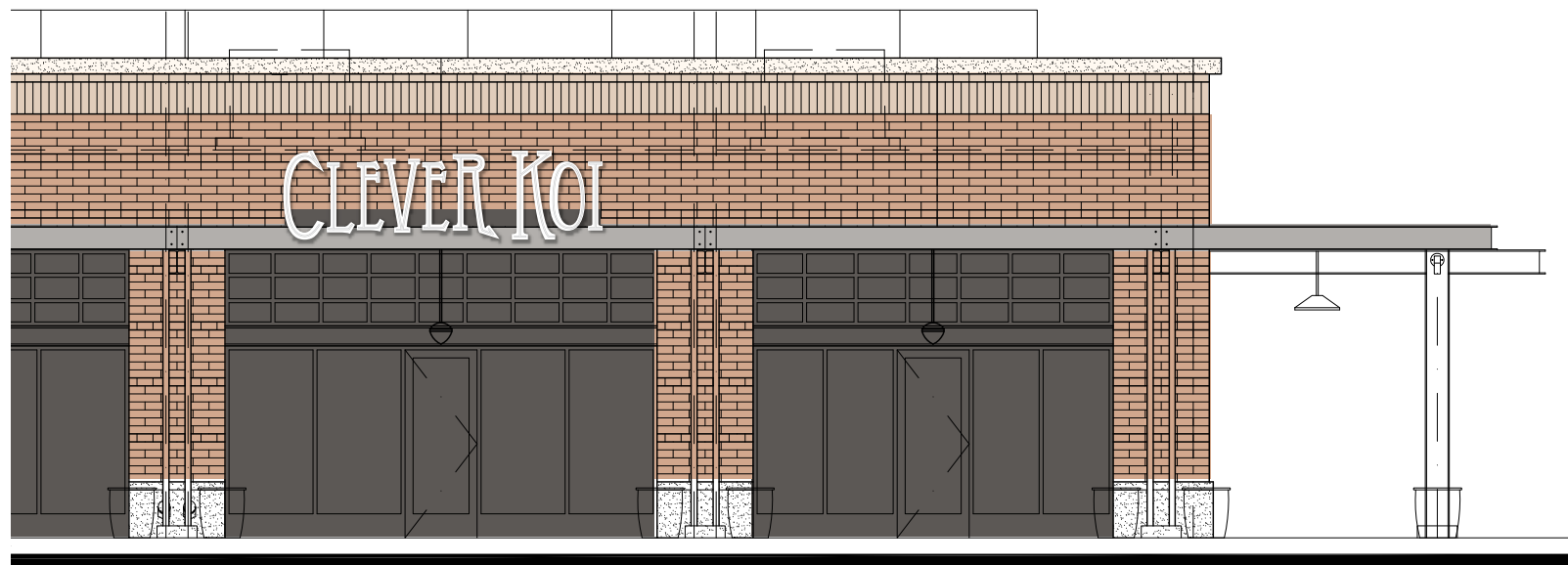
Canopy Mounted Sign with Exposed Raceway
