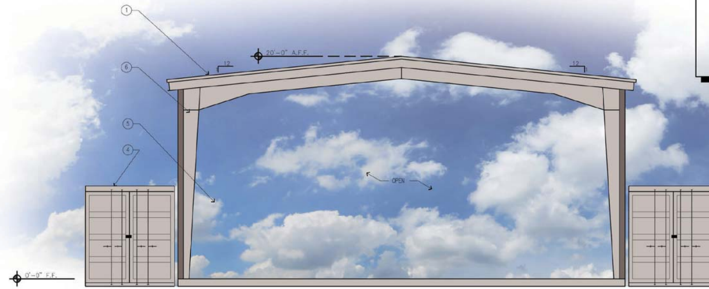
NORTH/SOUTH ELEVATION (WAREHOUSE) SCALE: 1/4" = 1'-0"
